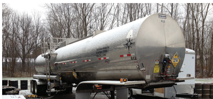
4,000 gallon mobile drop trailer with gravity feed and pump skid
